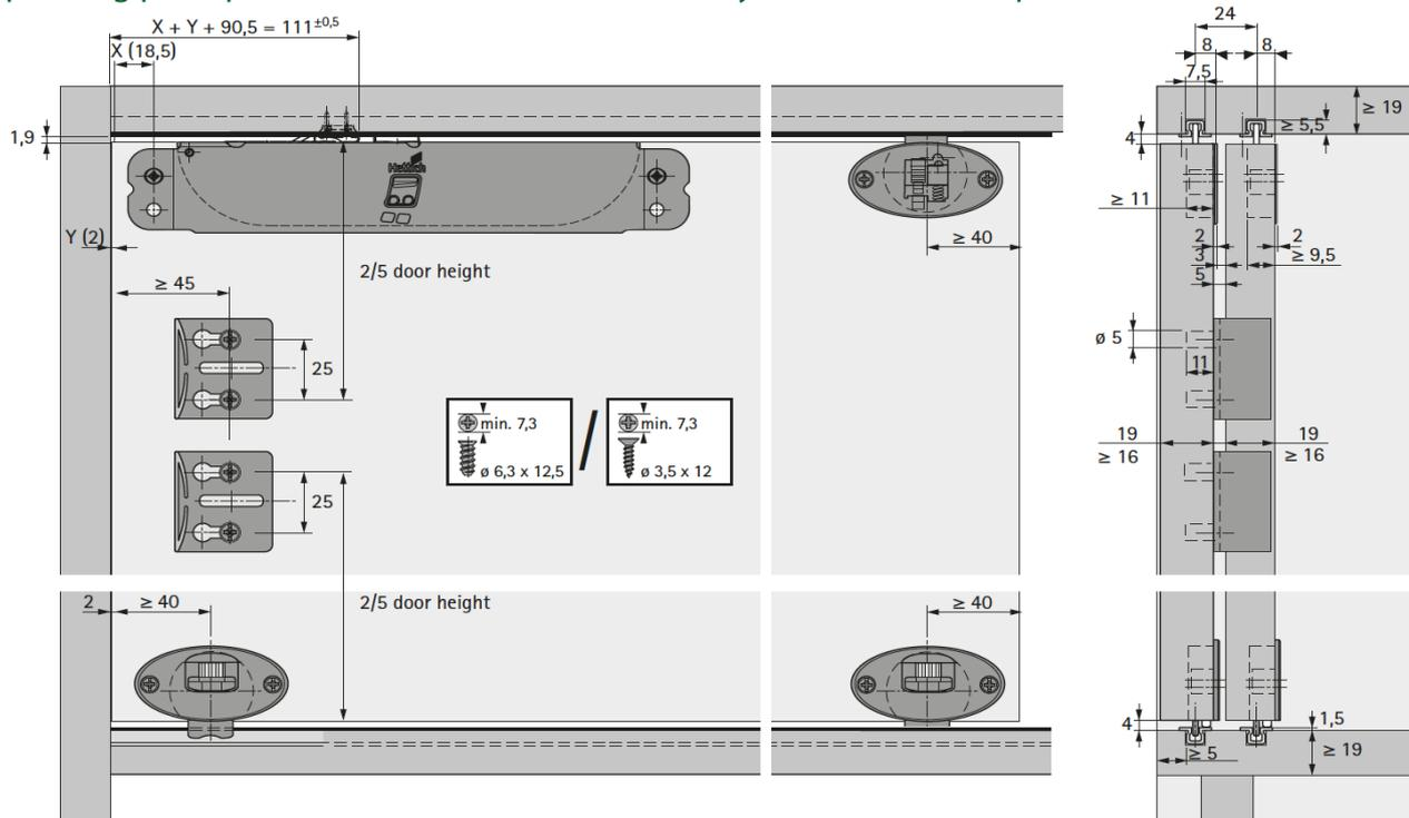
Operating principle / SlideLine 55 Plus with Silent System / overlay door position
