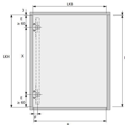
Recommended quantity of KA 5740 retractable door fittings depends on door height.
